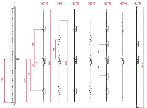
All door locks are twin spindle and accept shootbolts as standard (Dimensions in mm). Suitable for all front, back and french doors.
